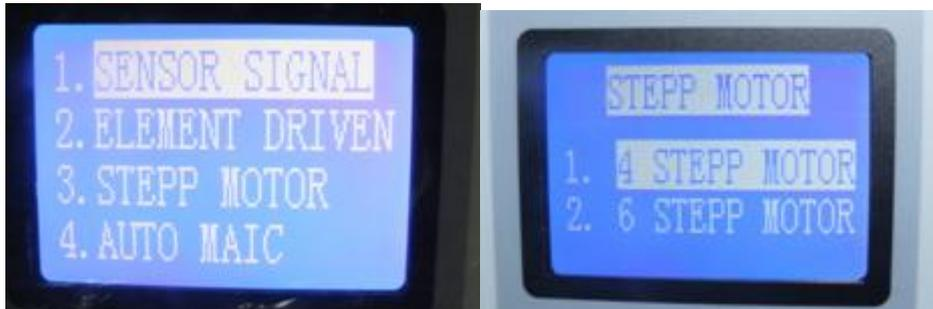
⑤ The fourth option, the entire vehicle simulation signal AUTO MAIC, select second option universal car signal simulation. ( or directly select F1, into the universal car signal simulation)
