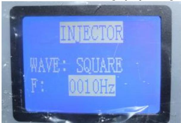
3, Simulation ignition driving signal output: choose SOLENOLD, +B,GND,PFC 3 port lamp shining after press RUN to enter, the analog signal ECU is PFC port, the port PFC signal output to ignition signal port, it can make the ignition drive for ignition, +and - for control of frequency and CYCLE.
