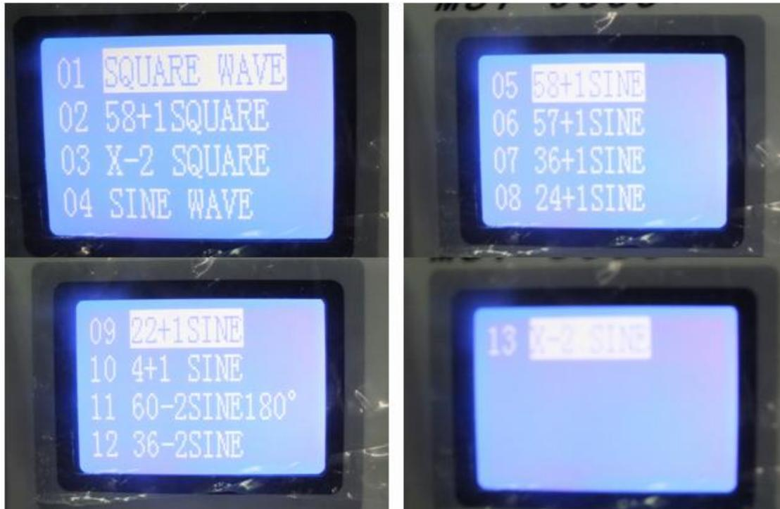
Select one ECU type to enter in, display change ECU output frequency (i.e.speed)adjustable range from 0020 to 2160 Hz, adjust by + and —, signal output end is +B (power), GND( ground wire), CKP (crankshaft speed signal), A1, A2, +,+,B1.B2, stepping motor signal output end.
