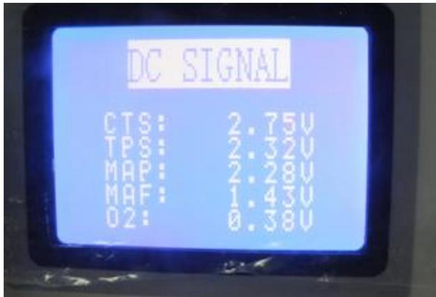
Displays on port CTS, TPS MAP, MAF, O2, +B, GND etc. will be blinking on those ports.
