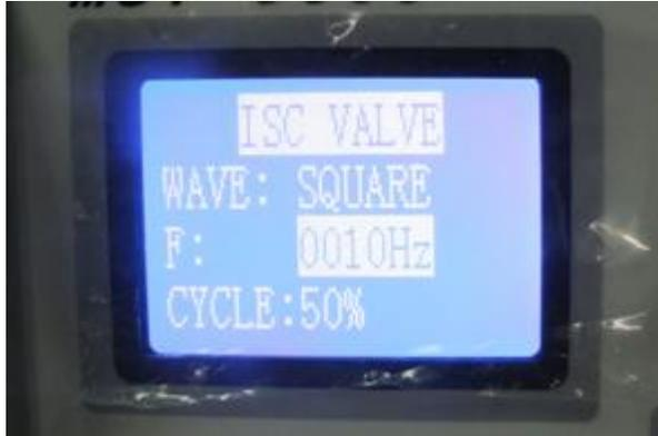
2, Simulation execution injection signal, choose INJECT, according to RUN after entering + B, GND, INJ, three port lamp shining, the analog ECU signal is INJ port, it connect to the nozzle, is nstrument sinmulation ECU signal control nozzle work, + and - can control injection instrument frequency, in the top of the instrument INJ - INJ6 six screen can display injection pulse width
